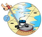
Bring 250 R.P.M. Powerhouse floor machine to area you will start. Strip floor with a black high productivity stripping pad.
