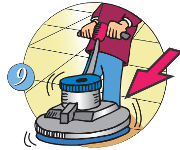
9 Once floor is dry, walk in a straight line at normal pace with a Cam Pro high-speed floor machine.
